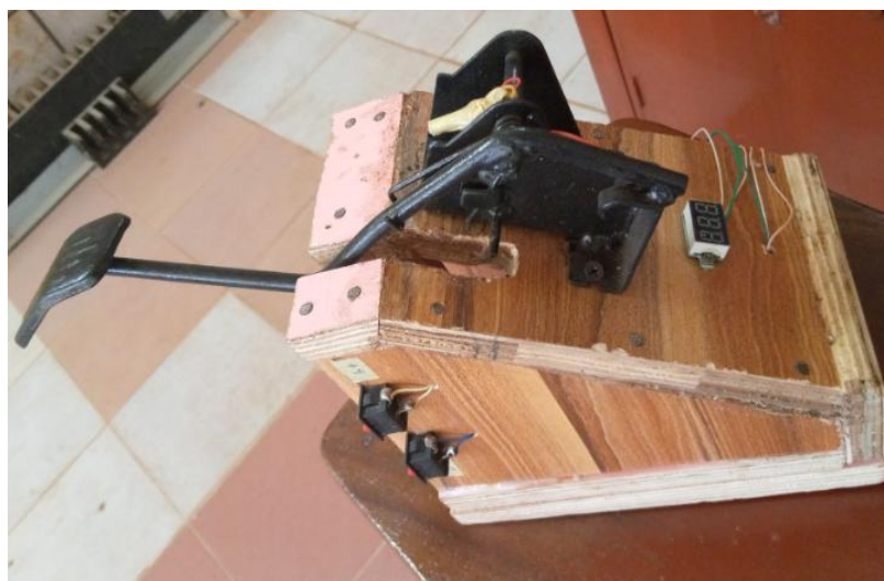
Fig.7: Side view of the accelerator pedal module
