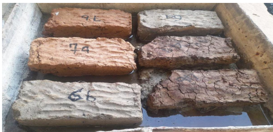
Figure 20. Failed sample during water absorption test
