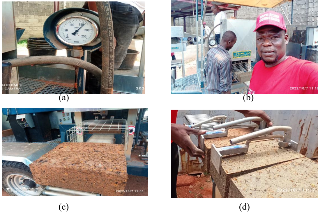
Figure 12. CEMB production (a) Pressure gauge, (b) Operation, (c) Typical CEMb and (d) Handle for carrying
