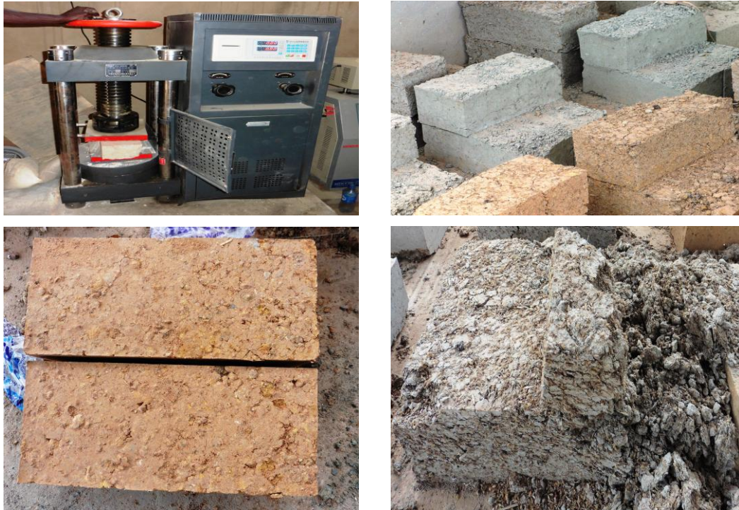
Figure 13. Compressive strength test (A) Compression machine, (B) Curing Bay, (C) Sample ready for weighing and crushing (D) failed sample which cannot be carried after curing, eg., some composite mix
