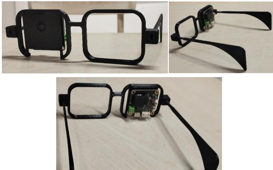
Figure 3: 3D Printed Indigenous AI Smart Glass
